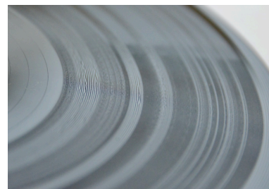
Figure 3.8: An extreme example of a disc in which the groove spacing has been varied to accommodate louder passages in the music. One consequence of this is that this side of the disc contains a single piece of music only 15 and a half minutes long.
