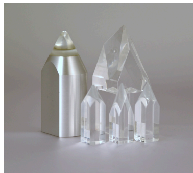
Figure 3.17: Scale models (on two different scales) of different styli. The example on the left is bonded, the other four are nude.
