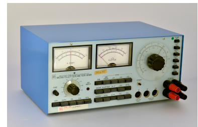
Figure 4.3: Bang & Olufsen WM1, analogue wow and flutter meter.
